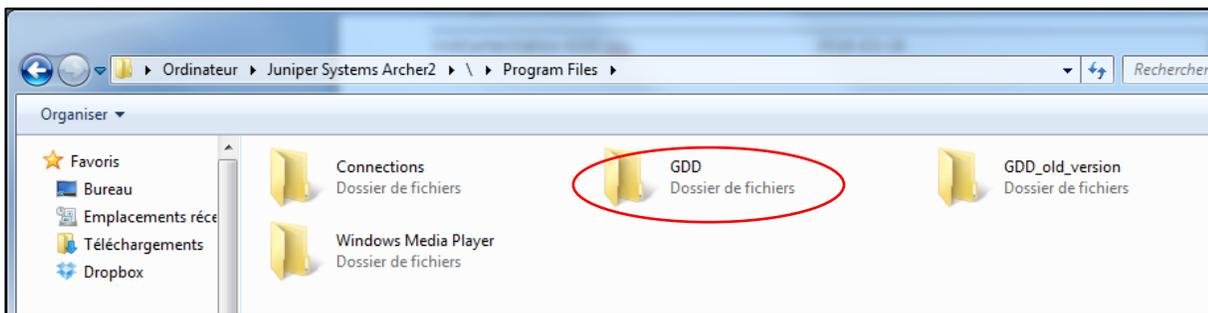
10. Use the drag and drop or the copy and paste functions to move the new GDD SCIP software files from your computer to your Archer<sup>2</sup> PDA's new GDD folder.
