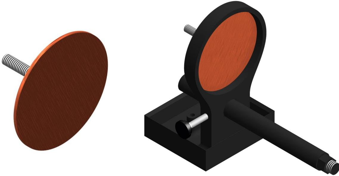
The electrode consists of a copper disc with a stainless-steel bolt. The banana connector can be inserted into the bolt for better contact. It is possible to adjust the distance between the electrode and the holder by screwing or unscrewing the electrode using the Allen key.
