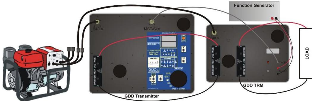
**Figure 2 - Wiring diagram for 1x GDD 5000W IP Transmitter and 1x GDD TRM configuration (up to 2400V / 5000W / 10A)**
