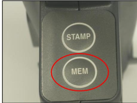
In this mode, each time you click **MEM** button in the GDD MPP software or you press **MEM** button on the probe, one reading is stored in the current project. This reading is associated to the selected **Core** and taken at the current **Depth** position. If the current **Spacing** is not **0**, the current **Depth** is incremented by the value of **Spacing** and the next reading will be stored at this **Depth** position.
