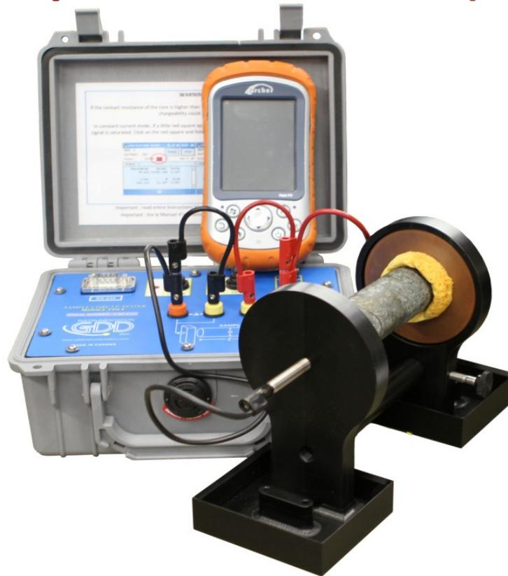
Get the information that you need to design an appropriate geophysical survey! **SCIP** is an innovative way to measure electrical properties of drill cores, hand samples or outcrops. Provides real time feedback. Relates DDH cores to resistivity and IP survey results. Allows constraining geophysical inversions.
