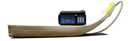
Enhance your geological mapping and prospecting campaigns by detecting sub-cropping Magnetic and Conductive bedrocks and floats. Follow-up on airborne EM anomalies and explain the shallow ones right away with a field visit.
