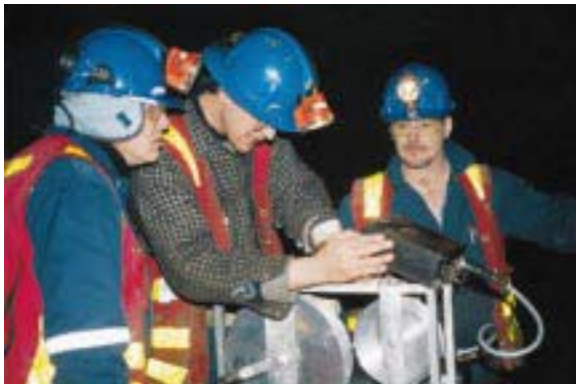
Fig. 4: Ron Lemery, Ken Germain and Mario Fluet at Raglan Mine are setting the new SSW system to verify ore contacts in their blast holes.
